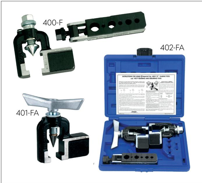
Forms 37° flares to government specifications in steel, stainless steel (including MIL-T-6845), titanium and other metal tubing. Positive stop gauge assures correct size of flare. Special burnishing action polishes flare face. Three rollers in flaring cone roll out 37° flare above die block. Roller action cuts effort required; maintains original wall thickness - eliminates stress concentration. Extension on yoke for clamping in vise. Satin chrome and black finish.
